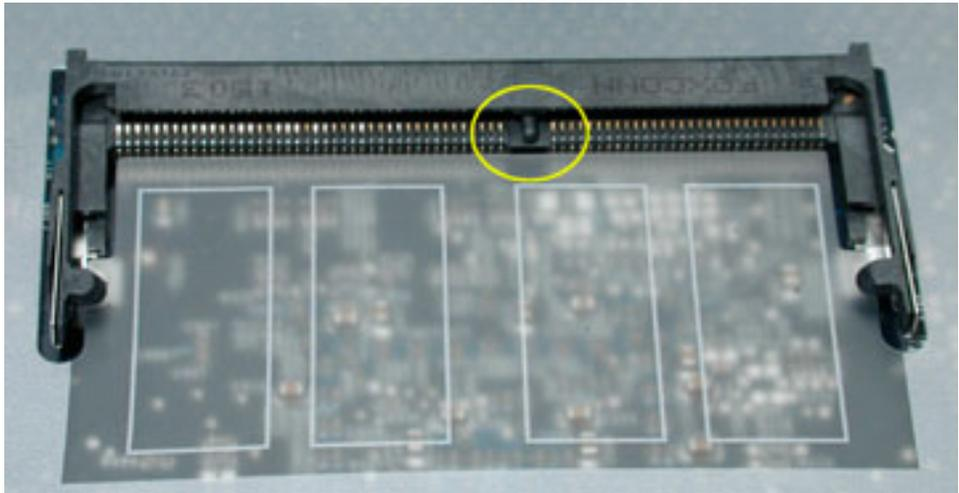
2. **Important:** Do not push the clips (circled below) when inserting memory. They are used to remove memory from the slot, not when inserting memory. These clips are fragile and can break.
