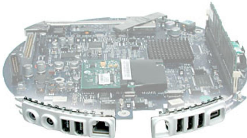
19. Replace the battery and memory on the logic board.
