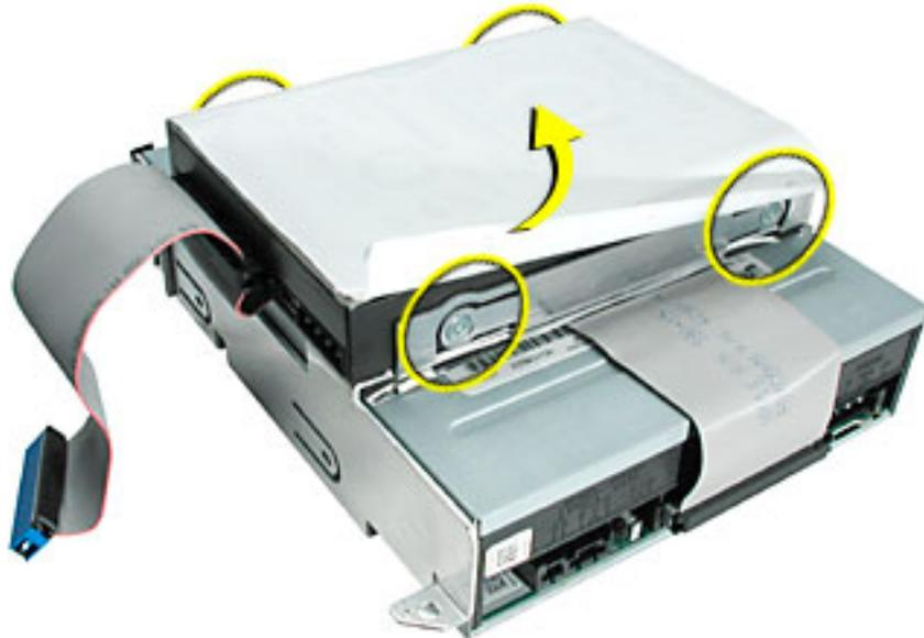
8. Remove the hard drive from the carrier.
