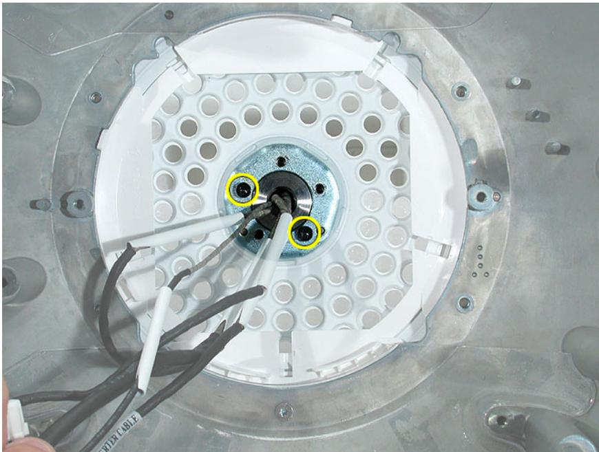
6. Route the neck cables in the base (as shown) and replace the three silver screws in the neck cap retainer.
