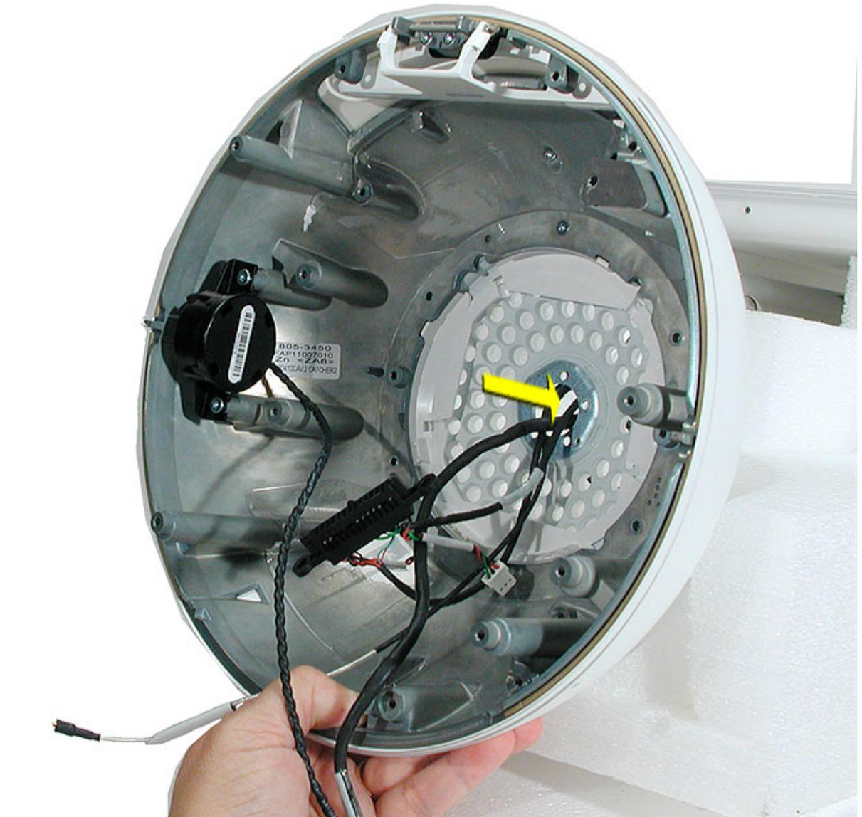
2. Pull the outer shell (with Faraday attached) away from the neck. **Note:** There is no need to remove the outer shell from the Faraday unless you are replacing the outer shell. **Important:** Be careful not to scratch the white paint on the inside of the housing shell and the metal neck plate (with holes).
