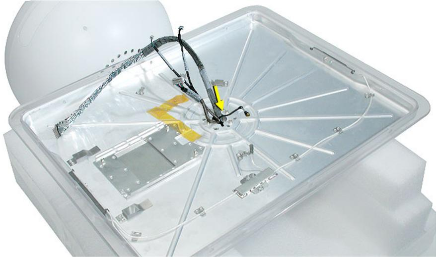
4. Line up the notches on the panel shield hole with the video cable. Gently pull the video cable through the panel shield (See next graphic for a close-up of the video cable going through the hole). Lift the shield off the back cover being careful not to scratch the white coating on the back cover.
