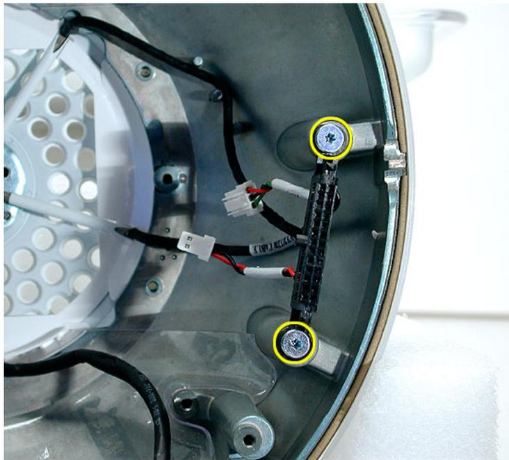
9. Attach the cable retainer and screws.
