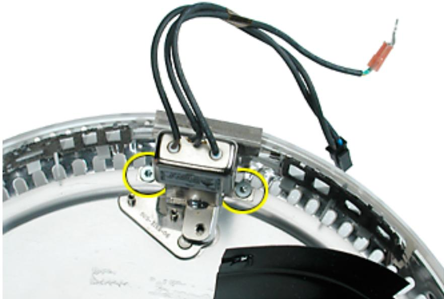
22. Replace the antenna extension and the black insulator into the bottom housing
