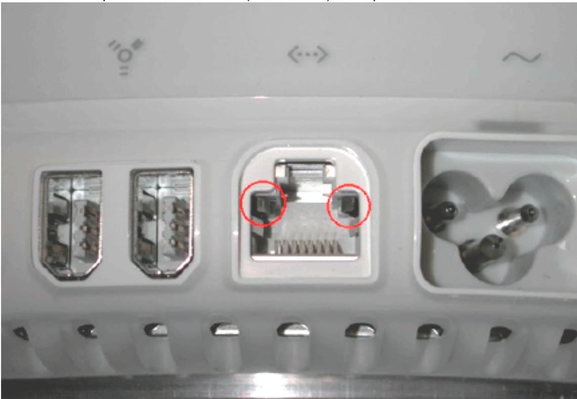
3. When inserting the Ethernet cable, try holding the cable at a slight angle and wiggle the connector to get past the metal tabs.
