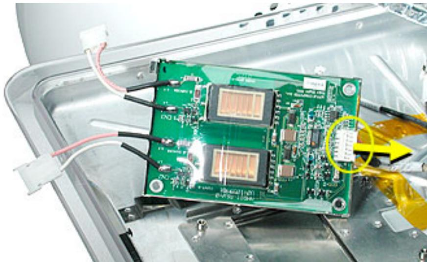
3. Remove the inverter from the display support shield.
