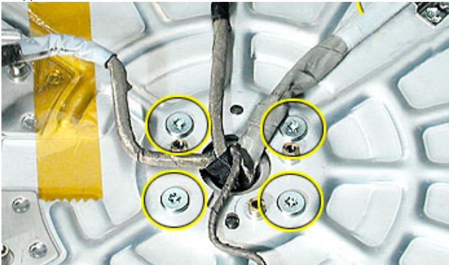
4. While holding the display bezel in this position, tighten the same four screws that hold the panel shield to the neck assembly.
