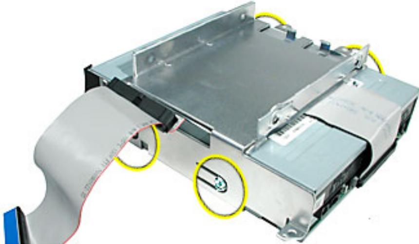
10. Slide the optical drive out of the carrier. Be careful of the black plastic dust filter on the carrier. It is very fragile and can rip easily if not handled properly. **Note:** The silver insulator is part of the carrier assembly.
