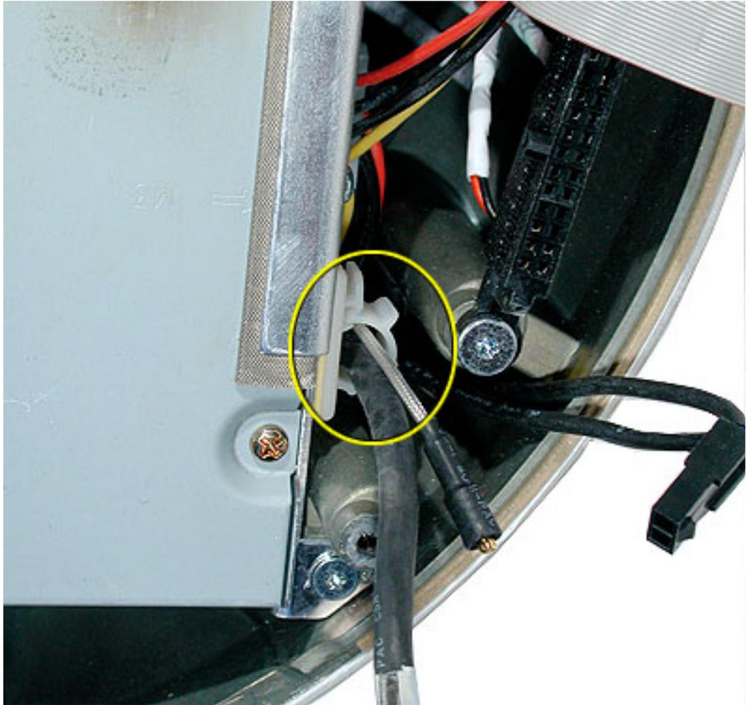
5. Grasp the carrier on both sides. Lift and pull the carrier in the direction of the arrow. Once the carrier is out, flip the carrier to the right to disconnect the power cables.
