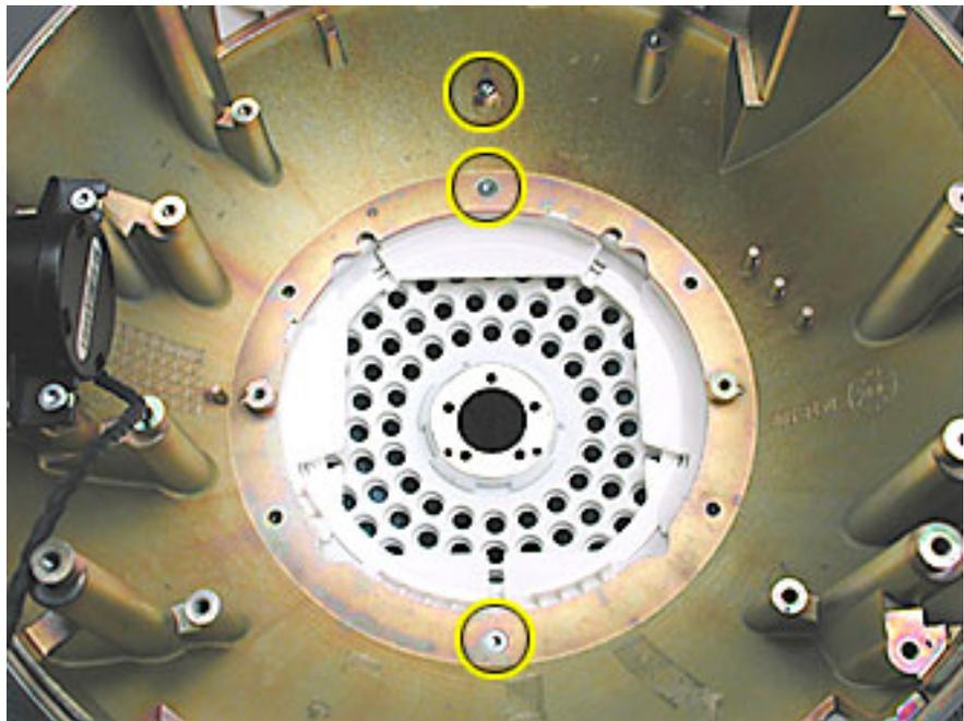
4. Thread the neck cables through the hole in the metal neck plate.
