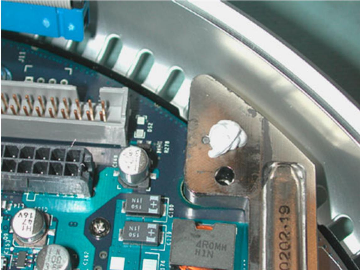
3. Close the bottom housing. Securely fasten the four mounting torx screws very firmly (at least 17 in.–lbs. is necessary). **Important:** If you don't have access to a calibrated torque driver make certain that the screws are tightened firmly. You don't need a torque driver; however, there is one available from Apple if you feel you need it. The torque driver part number is 076-0899.
