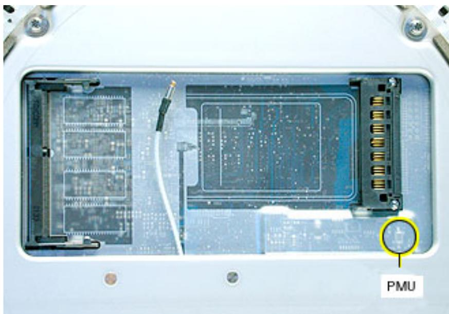
4. WAIT ten seconds before connecting the power cord and powering the computer on. If the computer powers on, go to the next step. If the computer does not power on, there is something else wrong with the computer, refer to the symptom/cure, “No Power” in this chapter.
