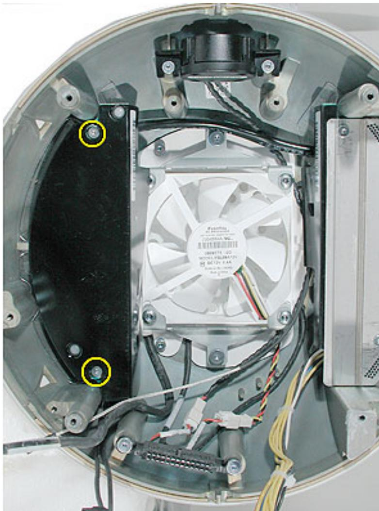
2. Open the optical drive door as shown to locate the two hidden screws near the drive door. Remove the four screws. **Note:** Support the metal plate and power supply as you remove the screws.
