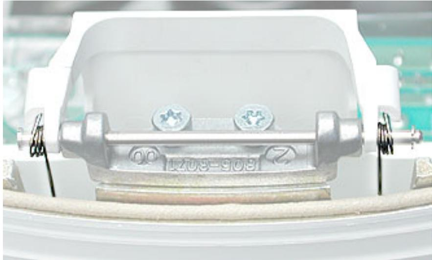
4. Remove the door hinge screws.
